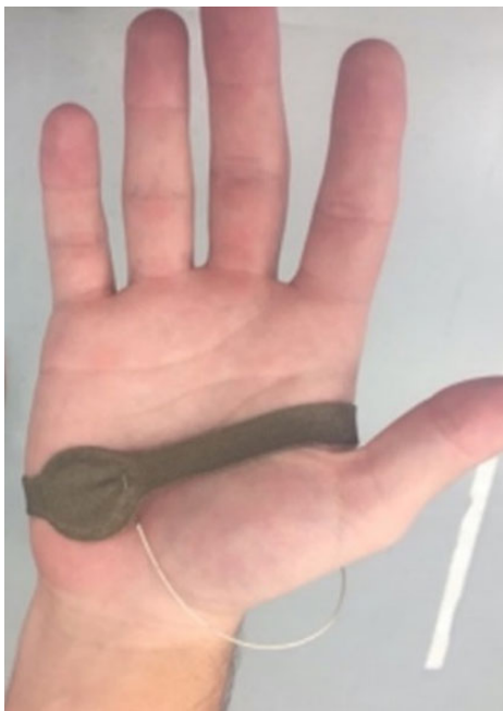
Figure 2. Experimental application of the FingerTPS Advanced Hand and Finger Pressure Sensor System to the hand.
